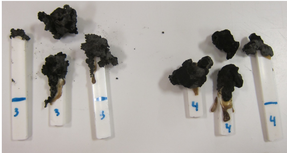
Char formation of 28% OrgNP-4 (left) and 24% OrgNO-4 + 1% Paxymer BGMB62 (right) after burning.
