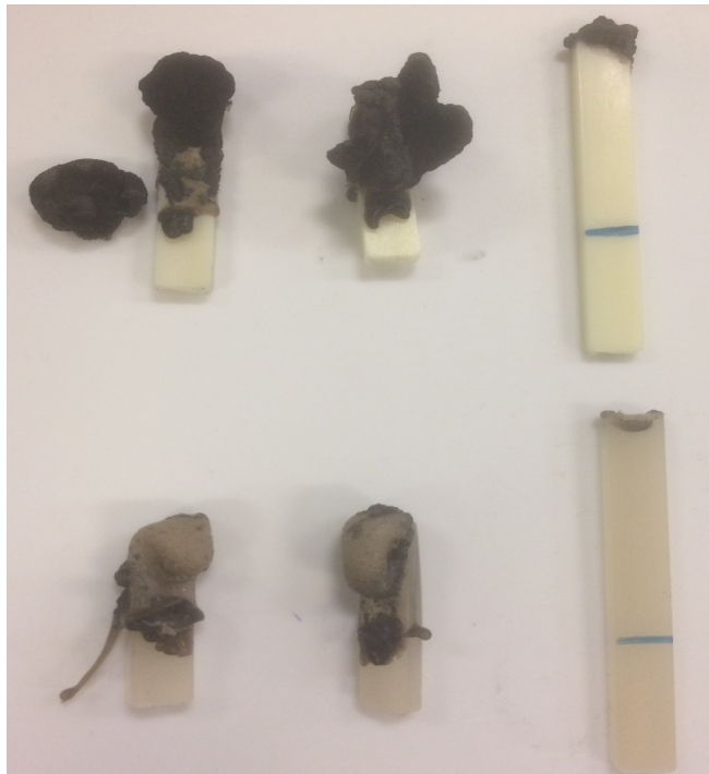
Char formation of 37% APP type II (top) and 25% APP-3 + 2% Paxymer BGMB62 + 5% N synergist (bottom) after burning.
